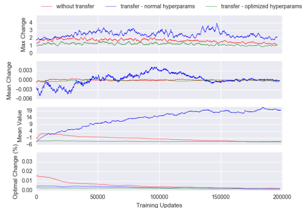
Figure 8: Convergence metrics during training over transfer and control networks. From the top: (1) maximum change in Q-value between updates (2) mean change in Q-value between updates (3) mean Q-value during training (4) percent change in optimal action between updates.
